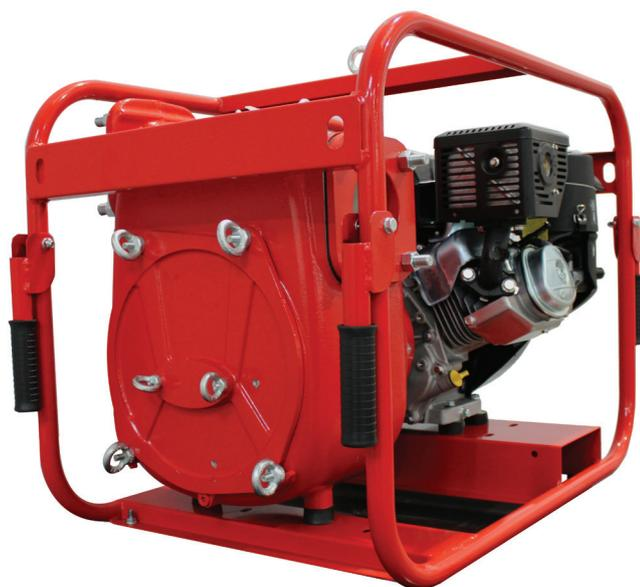
The self priming pump “Trash” is designed to comply to the hardest and heavy duty applications especially for emergency when there is dirty sewage and muddy water with the presence of solids and sand. The open-blade impeller ensures a superior priming ability voiding the need of a foot valve installation. The high thickness of the pump body and of the impeller blades, allow the handling of more abrasive fluids and large passage of solids.
